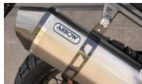
TITANIUM ARROW SILENCER 2.1 KG LIGHTER
