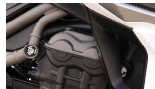
MAGNESIUM CAM COVER 0.3 KG LIGHTER
